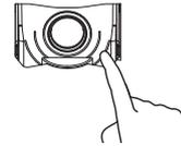
Adjust the orientation of the motion sensor by pressing the end of the sensor.
