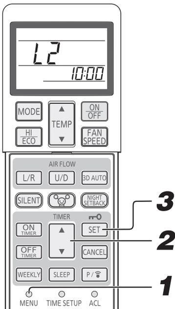
**1** Select the display brightness adjustment by pressing the MENU switch.
