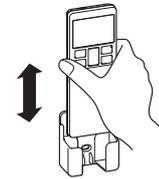
For installing or removing the remote control, move it up or down in the holder.
