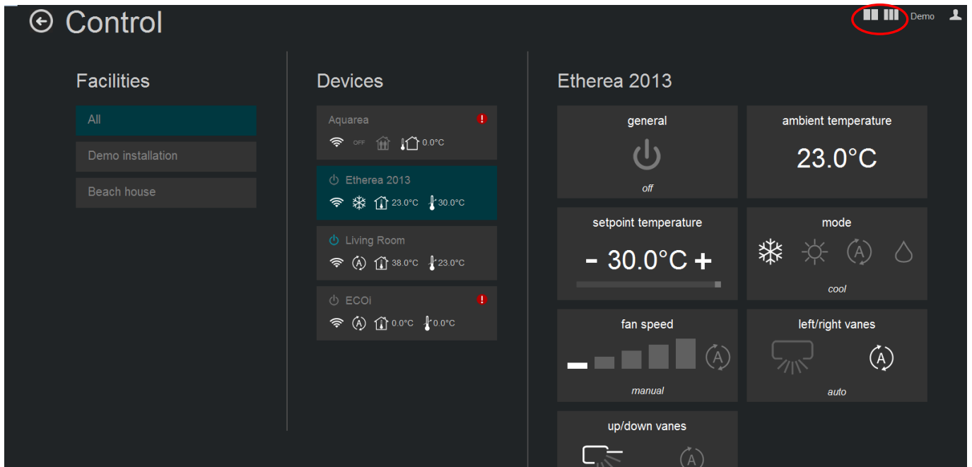
Figure 8-3 IntesisHome control interface (expanded)
